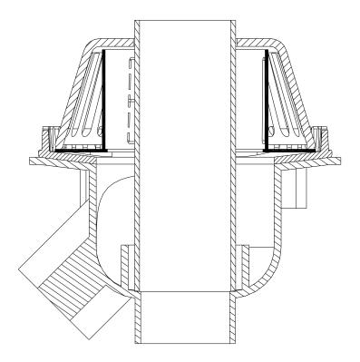
The Froet Drain® roof drain with control flow weir can be configured on the job site for the required amount of flow needed. The weir is produced with one weir open. The 3" and 4" bodies have 6 possible weir openings and the 5' and 6" bodies have 8 possible openings. The chart shows the flow thru one weir opening. The design of our weir also allows for removal of the weir assembly from the drain to facilitate cleaning a plugged drain or piping without breaking the seal with the roofing membrane.
