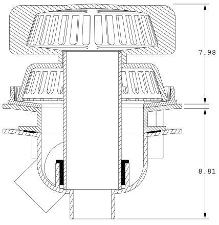
Please Note: The Gasket supplied with the extension must be installed to provide watertight installation.
