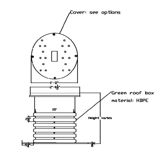
PLEASE NOTE: The HDPE adjustable green roof box will only accommodate the 2" thru 6" 100 series drains, the 3" thru 6" 200 Series drains and 5" thru 8" 200LD series drains
