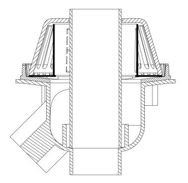
The Froet Drain® roof drain with control flow weir can be configured on the job site for the required amount of flow needed. The weir is produced with one weir open. The 3" and 4" bodies have 6 possible weir openings and the 5'and 6" bodies have 8 possible openings. The chart shows the flow thru one weir opening. The design of our weir also allows for removal of the weir assembly from the drain to facilitate cleaning a plugged drain or piping without breaking the seal with the roofing membrane.
