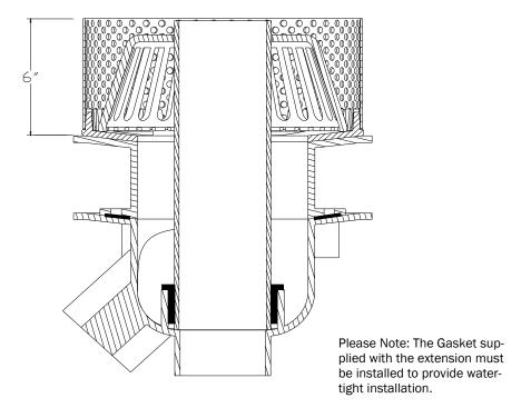
Please Note: The use of the IRMA Guard with a conventional roof system will restrict small debris that would normally pass thru the drainage system. This will block the IRMA Guard and will require increased frequency for maintenance.
